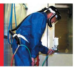
The 3M Supplied Air Visor System - AL4P features an air regulating valve and acetate nod down painting shield with foam face seal. An optional Y-piece take off (shown) may be fitted allowing the use of one airline hose to provide air for respiratory protection and spray gun.
