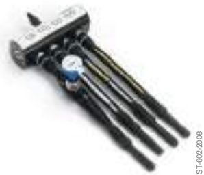
Impactor with Adapter in Aerotest Simultan
