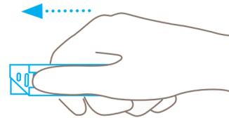
Use the slider to **engage the blade** for cutting.
