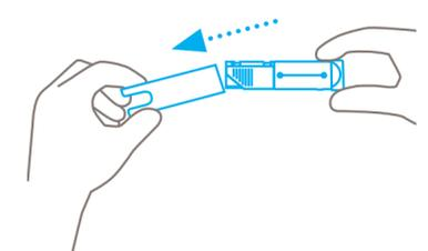
Finally, re-insert the plastic insert and blade **fully into the handle**.
