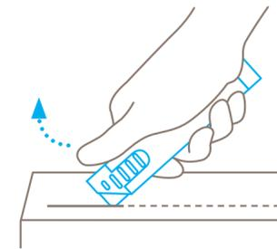
Always remove your **thumb from the slider** to ensure automatic blade retraction.
