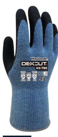
WG-780 Dexcut™ is a nitrile coated cold-resistant glove that also offers high cut resistance (ISO 13997 grade D), thanks to its 10-gauge acrylic pile liner mixed with aramid and mineral fibre. Our SNZT™ engineered nitrile coating WG-780 remains flexible in sub-zero temperatures, down to -20 °C. WG-780 Dexcut™ is a unique glove for users seeking a glove able to keep the hands warm while protecting them from cuts, making it the ideal choice for outdoor winter work.
